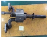
Secondary nozzle before repair
