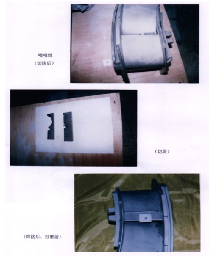
Primary nozzle repairment of Gas Turbine MS6001B Mode
