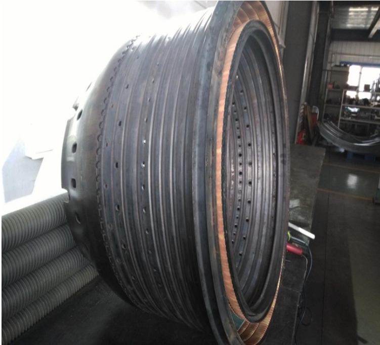
Combustion chamber repairment of Gas Turbine LM2500+SAC
