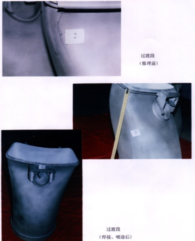
Transition section repairment of Gas Turbine MS5001B Mode
